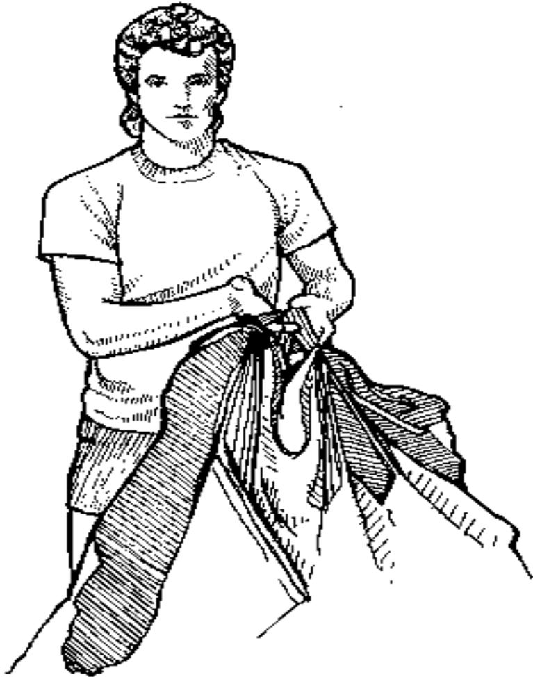
5) The nose openings should be facing the rig and the tail should be farthest from the rig. If the reverse is true, double check to be sure the rig is container-side up (the back pad is on the ground). If the rig is positioned correctly and the canopy is not oriented as described above, then the canopy was attached to the harness backwards!
