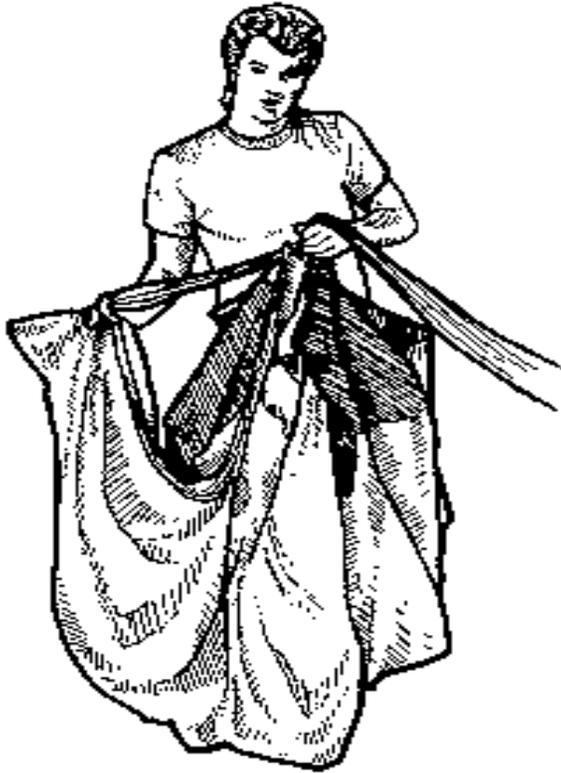
25) Now grasp the steering lines where they attach to the tail, pull the entire tail out and drop it straight down.
