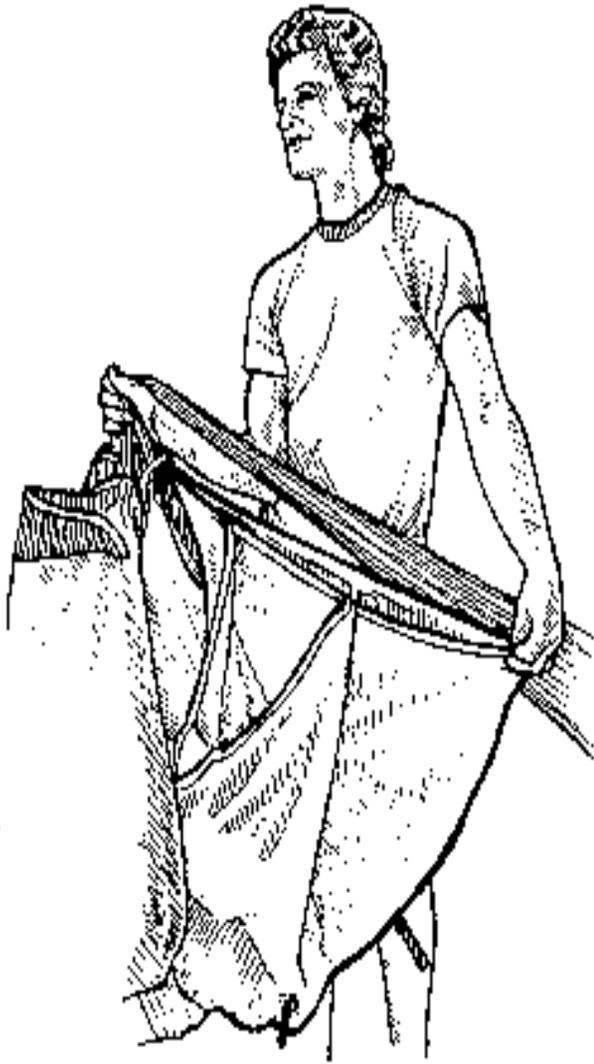
7) Starting with the end cell nearest your legs, flake the entire nose with one hand as shown.
